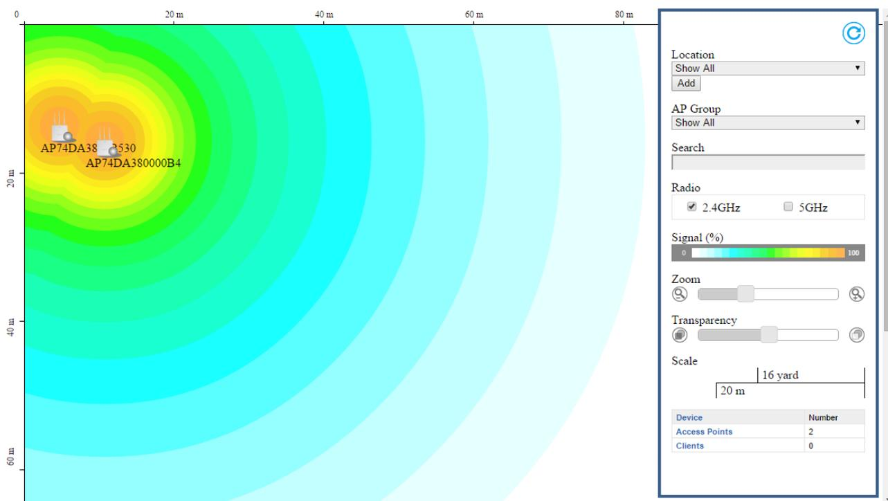
**Zone Plan** displays a customizable live map of Managed APs for a visual representation of your network coverage. Each AP icon can be moved around the map, and a background image can be uploaded for user-defined location profiles using **NMS Settings** → **Zone Edit**. Options can be configured using the menu on the right side and signal strength is displayed for each AP.
