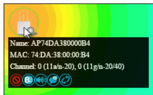
Click and drag an AP icon to move the icon around the zone map. The signal strength for each AP is displayed according to the “Signal” key in the menu on the right side:
