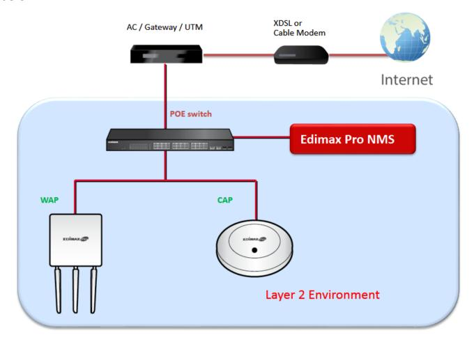
One AP (access point) is designated as the AP Controller (master) and other connected Edimax Pro APs are automatically designated as Managed APs (slaves). Using Edimax Pro NMS you can monitor, configure and manage all Managed APs (up to 8) from the single AP Controller.
