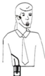
To use a "Lavalier" microphone connect the jack at the transmitter input and move the selector to L.
